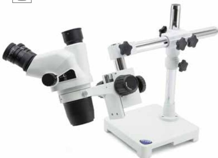
Trinocular stereomicroscope with extremely stable overhanging stand complete of head holder and focusing system for perpendicular observation of particularly large specimens. Smooth horizontal and vertical movements are ensured. In case illumination is needed, choose from the wide choice of external illuminators available.
