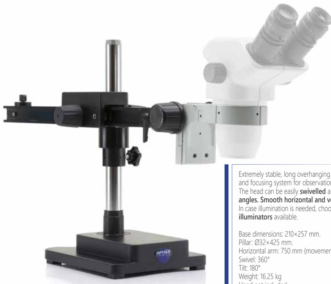
Extremely stable, long overhanging stand complete of head holder and focusing system for observation of particularly large specimens. The head can be easily **swivelled** and **tilted** for inspection at **oblique angles**. **Smooth horizontal and vertical movements** are ensured. In case illumination is needed, choose from the wide choice of **external illuminators** available.
