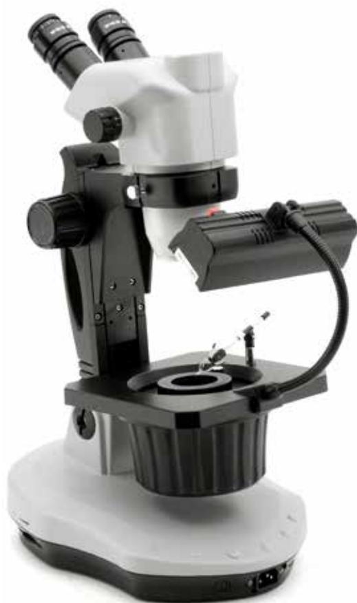
Binocular gemological stereomicroscopes for brightfield and darkfield applications. The darkfield condenser uses a typical optical configuration, based on halogen illumination and a classic reflecting system. A flexible arm with a fluorescent tube simulates the color of daylight for accurate color grading. The stand can be inclined backward by 45° for to increase comfort and ergonomoy.
