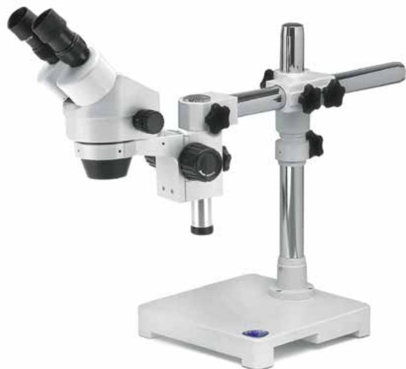
Binocular stereomicroscope with extremely stable overhanging stand complete of head holder and focusing system for perpendicular observation of particularly large specimens. Smooth horizontal and vertical movement are ensured. In case illumination is needed, choose from the wide choice of external illuminators available.
