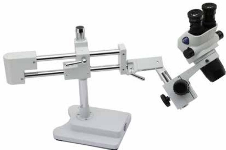
Binocular stereomicroscope with extremely stable, hinged and long overhanging stand complete of head holder and focusing system for observation of particularly large specimens. The head can be easily tilted for inspection at oblique angles ideal e.g. for stone setters. Smooth horizontal and vertical movement are ensured. In case illumination is needed, choose from the wide choice of external illuminators available.
