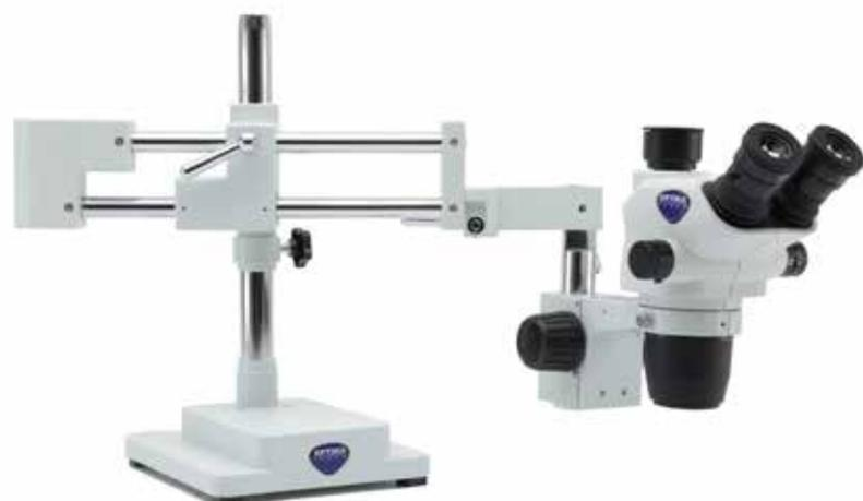
Binocular stereomicroscope with extremely stable, hinged and long overhanging stand complete of head holder and focusing system for observation of particularly large specimens. The head can be easily tilted for inspection at oblique angles ideal e.g. for stone setters. Smooth horizontal and vertical movement are ensured. In case illumination is needed, choose from the wide choice of external illuminators available.
