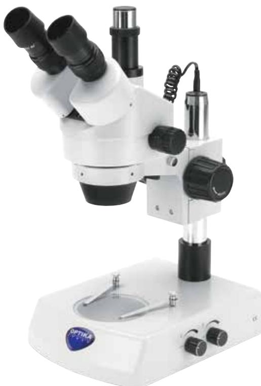
Trinocular stereomicroscope with pillar stand and illuminated stage with halogen transmitted and incident illumination, freely settable.
