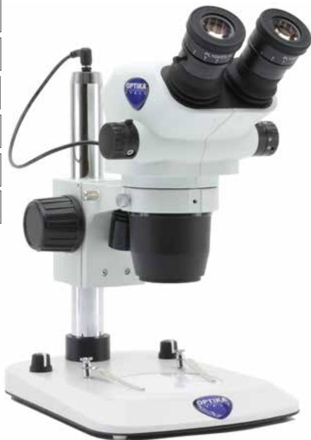
Binocular stereomicroscope with pillar stand and ultra-flat base, illuminated stage with **X-LED<sup>73</sup>** transmitted illumination and **X-LED<sup>3</sup>** incident illuminator for outstanding brightness, freely settable.
