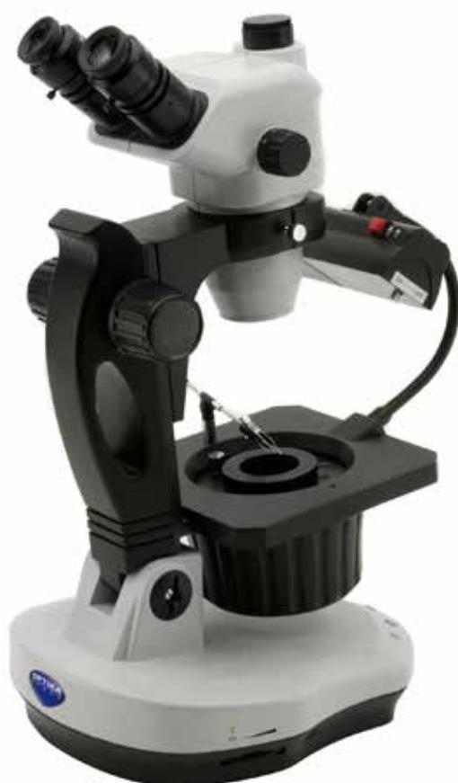
Trinocular gemological stereomicroscopes for brightfield and darkfield applications. The darkfield condenser uses a typical optical configuration, based on halogen illumination and a classic reflecting system. A flexible arm with a fluorescent tube simulates the color of daylight for accurate color grading. The stand can be inclined backward by 45° for to increase comfort and ergonomoy.
